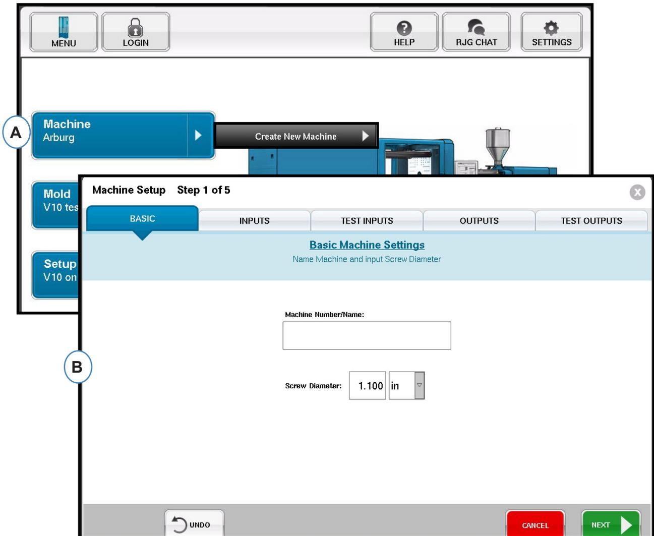
**A:** Select the Machine button on the eDART Home page, then select the Create New Machine button.
