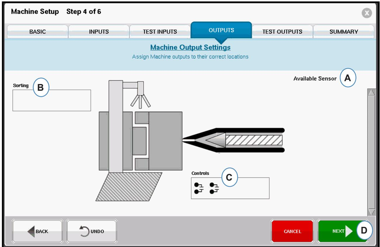
**A:** Drag Output Modules from the Available Sensor list into the correct location.
