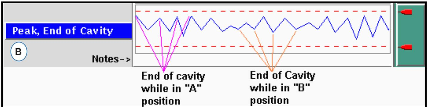
**B:** Fixed Half Sensors—Fixed half sensors plot a data point on every shot. If the mold shuttles from shot to shot, it is possible to see the alternate data between two halves.
