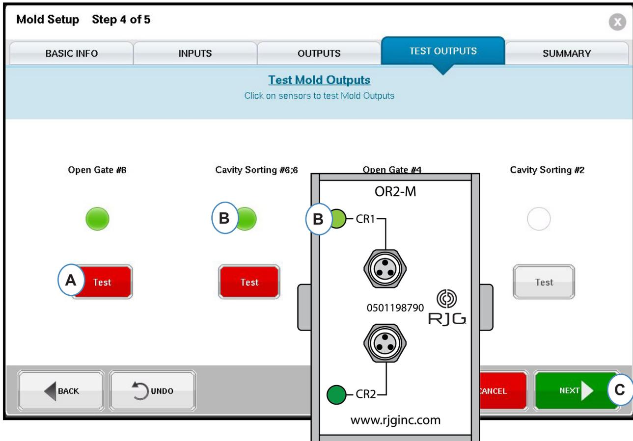
**A:** Select the Test button to individually test each available output.
