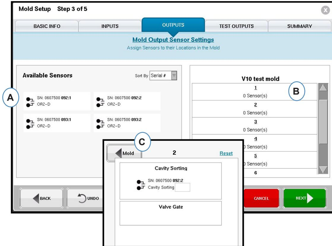
**A:** Drag a sensor from the Available Sensor list on the left and drop into the correct cavity on the right.
