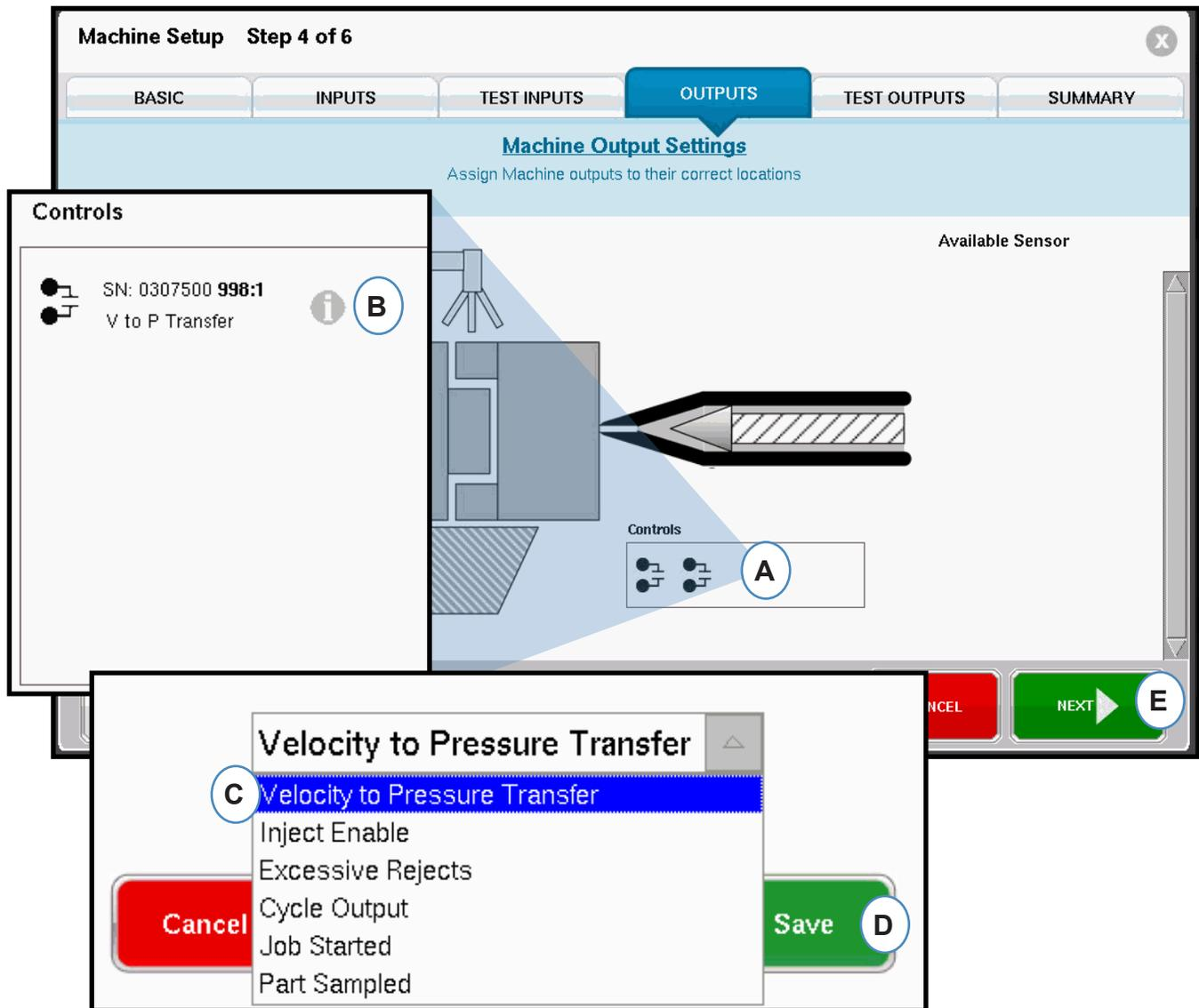
**A:** Drag a module from the Available Sensor list to the Control box, and drop in the correct location.
