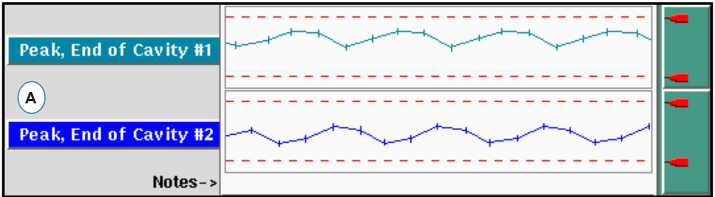
**A:** Moving Half Sensors—One sensor is active while one sensor is inactive; data points therefore will alternate for each mold half.
