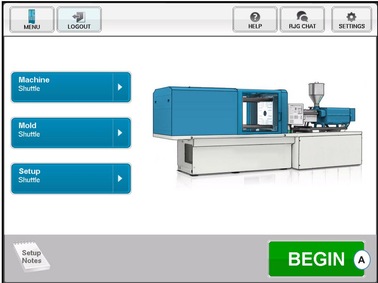
**A:** Once the machine, mold, and process are set up, select the BEGIN button to start the job.
