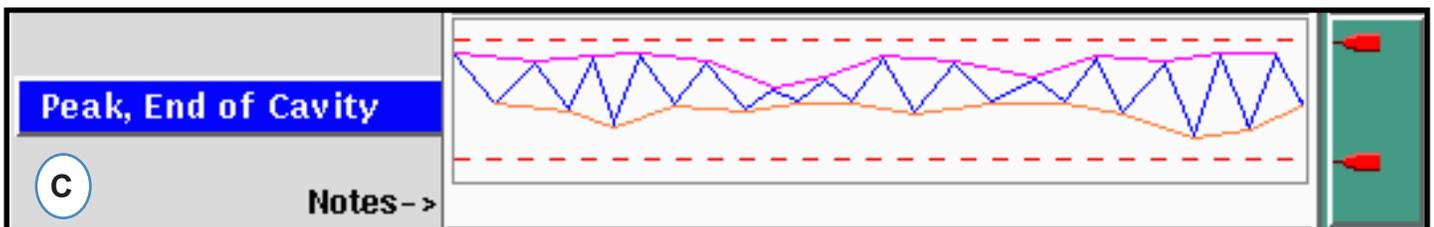
**C:** Fixed Half Sensors—The upper and lower lines show the data trend for each mold half (these lines are for illustration only— lines are not plotted by the eDART).
