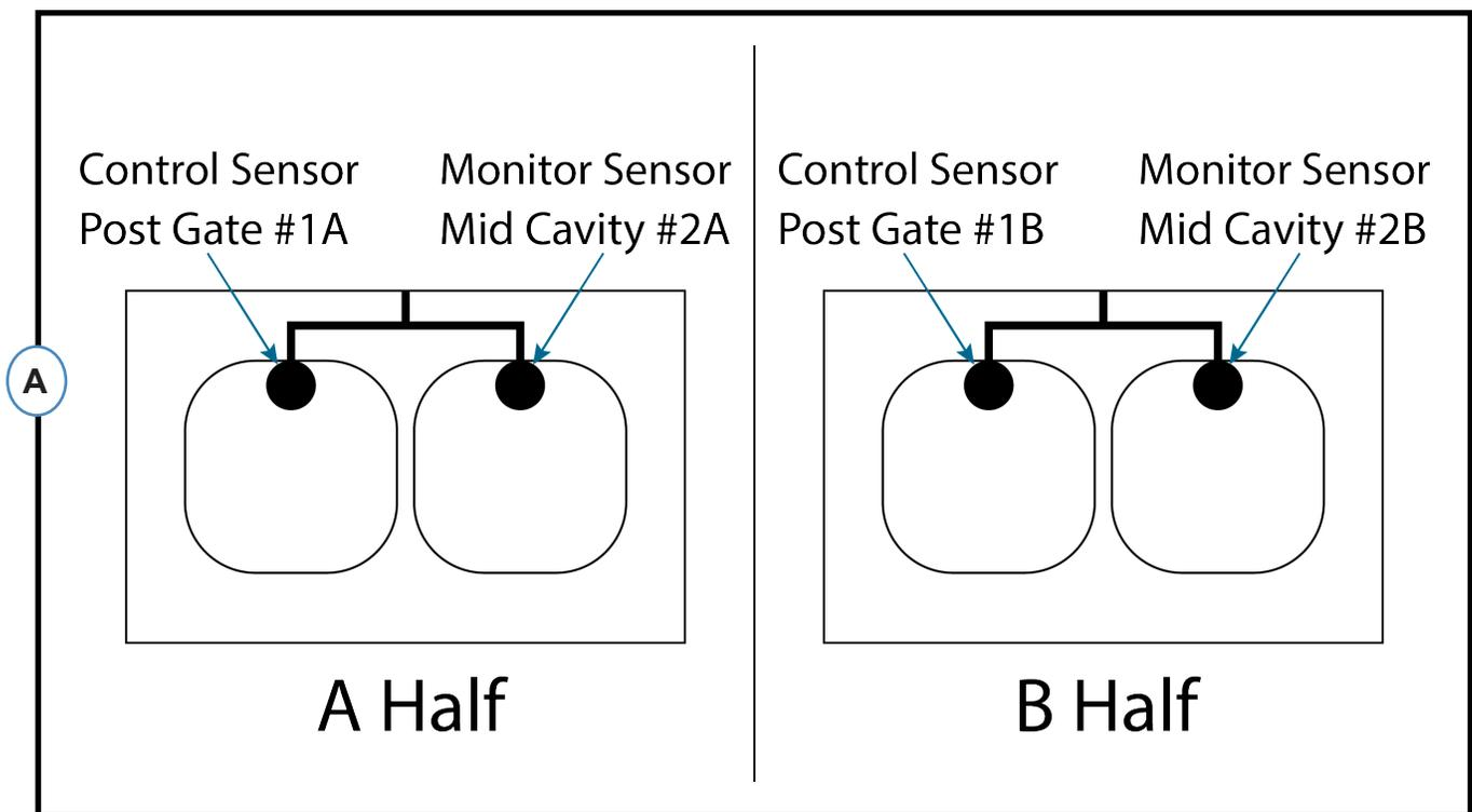
**A:** To set up V→P control from a specific sensor in a multi-cavity mold with multiple sensors in the same location, the non-control sensors must be designated as a different location than the controlling sensor. For example, the control sensor is designated as Post Gate; the remaining sensors are designated as Mid Cavity—even if the non-control sensors are located Post Gate.
