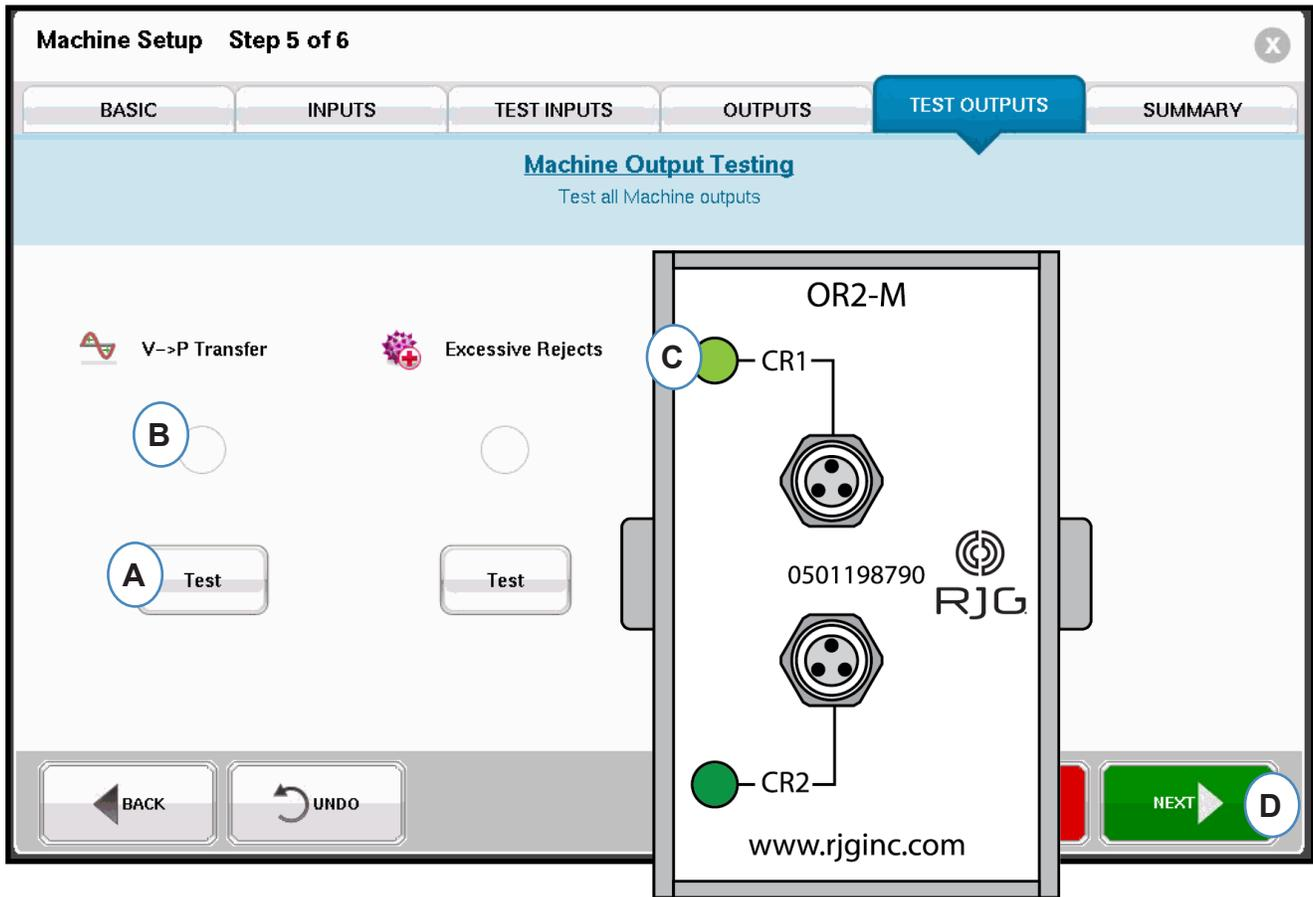
**A:** Select the Test button to individually test each available output.
